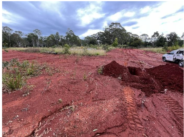
TP12- Looking at the intersection of Road 8 and Road 9 that is underlain by red residual clay.
